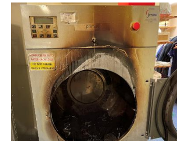
Figure 5 Tumble dryer following a sprinkler save in Wellingborough care home ©NFRS
