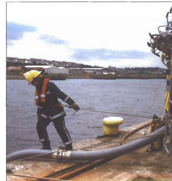
Figure 2.3 A pump operator at dockside in work restraint.
