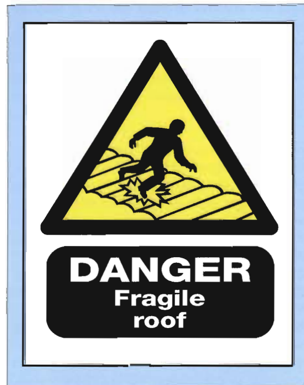
Figure 2.58 Typical fragile material warning sign.
