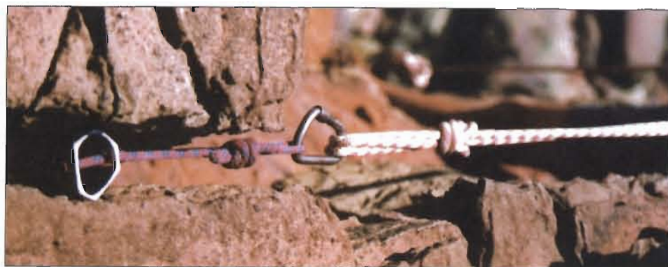
Figure 2.39 Photograph of climbing equipment in use as temporary artificial anchor.
