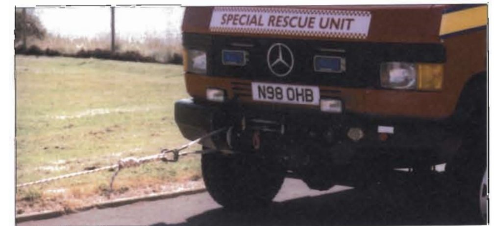
Figure 2.38 Photograph of vehicle being used as a temporary artificial anchor.
