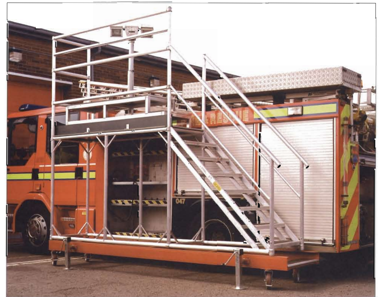
Figure 2.59 Access steps and working platform for vehicle maintenance.
