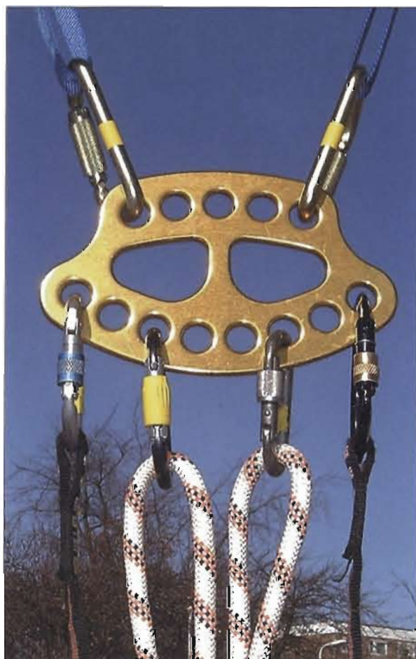
Figure 2.28 Photograph of a rigging plate in use.
