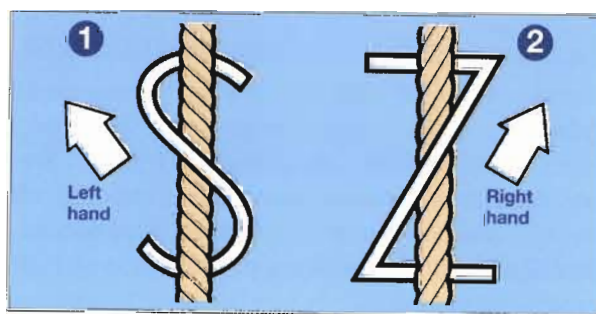
Figure 3.3 Diagram showing hawser laid rope in traditional 'S' and 'Z' lays.
