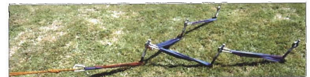
Figure 2.37b Photograph showing V-configuration of ground anchor system.
