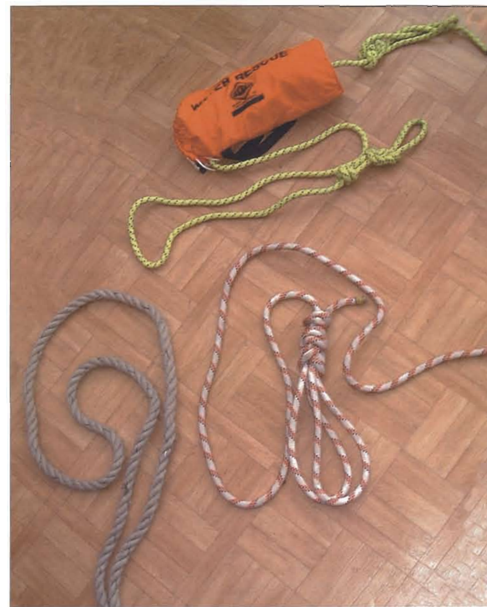
Figure 3.6 Photograph showing a variety of types of rope and cordage including kernmantel rope; British Standard 16mm hawser laid polyester GP line and an example of floating rope.
