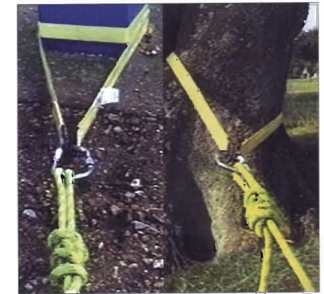
Figure 2.27 Photograph of temporary artificial anchors.
