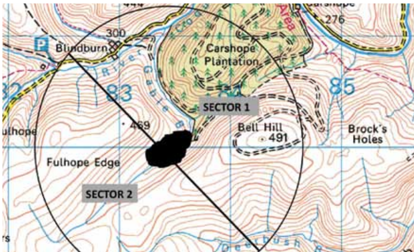
◀ Fig. B7.14 The landscape can now be sectored in a number of ways. This example shows that the fire has been divided into two sectors. Sector 1 covers the area in which the head part of the fire may expand into. Sector 2 covers the area in which the flanks and tail may develop.
