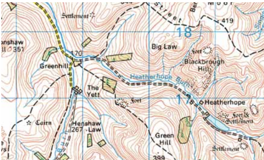
Fig. B3.8 An example of how valleys are shown on a map
