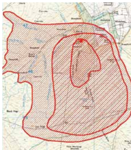
Fig. B6.14 Showing the potential fire spread over a 6-hour period
