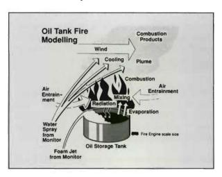
It has also been suggested that projection of water sprays into the 'plume' of flame and hot gases rising from the tank may cool the plume significantly and allow more foam to reach the oil surface.
