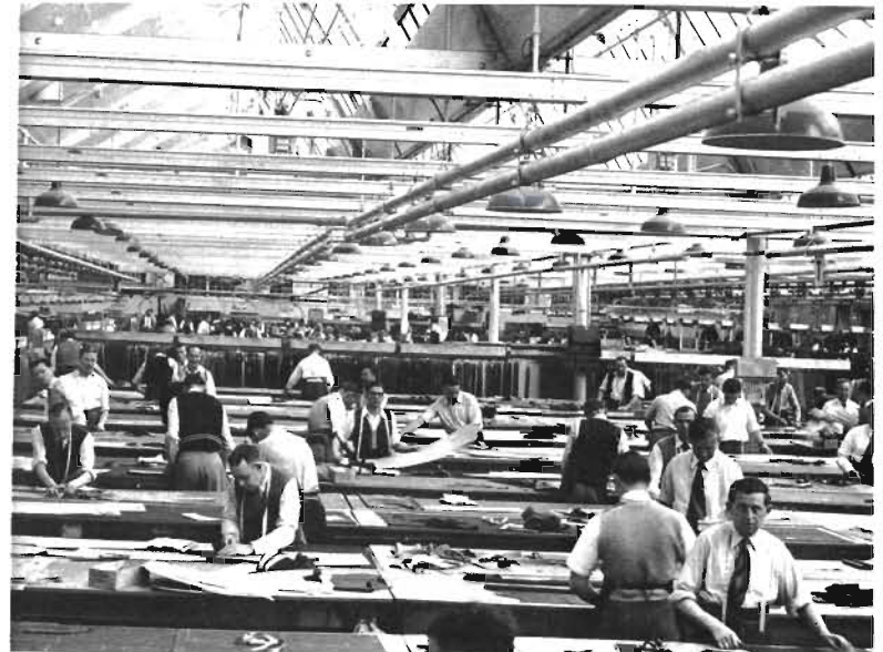
Plate 23. The cutting room of a modern clothing factory. Note the large amount of stock in the background which is liable to lose much of its value if wetted. (Section 4).
