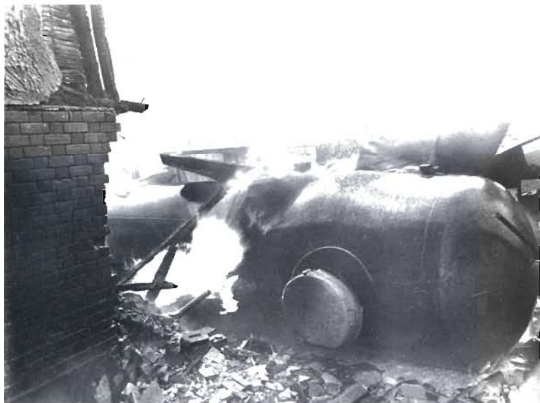
Plate 26. A close-up of the overturned tanker shown in Plate 25; the butane is burning at the points of fracture. The pressure bulges which developed in the tank can be clearly seen. (Section 5).
