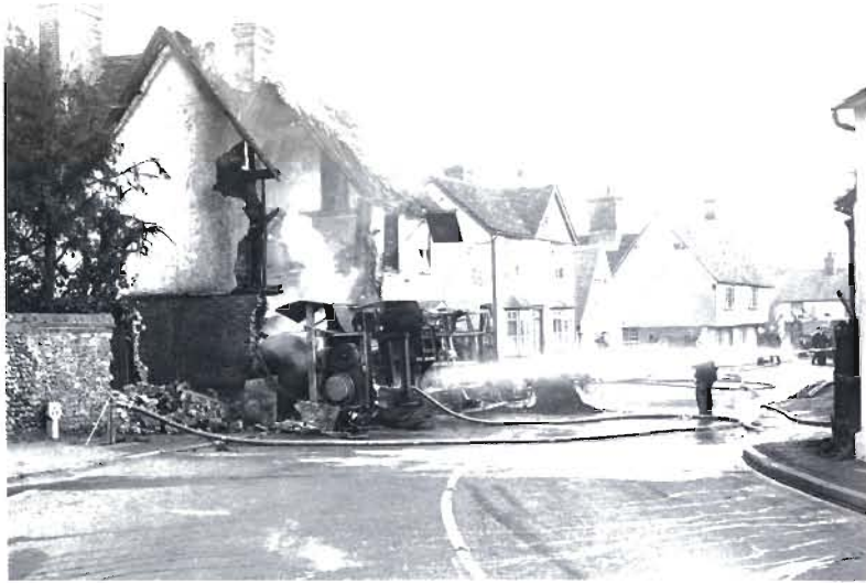
Plate 25. A road tanker carrying 5586 kg of liquid butane, which overturned on the road. The gas escaping from the fractured tank ignited immediately. (Section 5).
