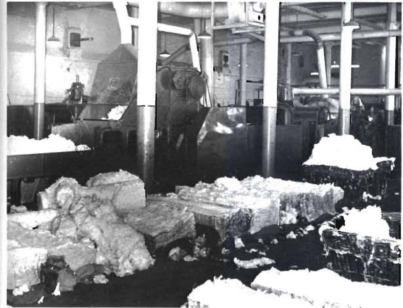
Plate 12. Bales of cotton being opened up prior to being fed into the breaking or opening machines. (Section 4).
