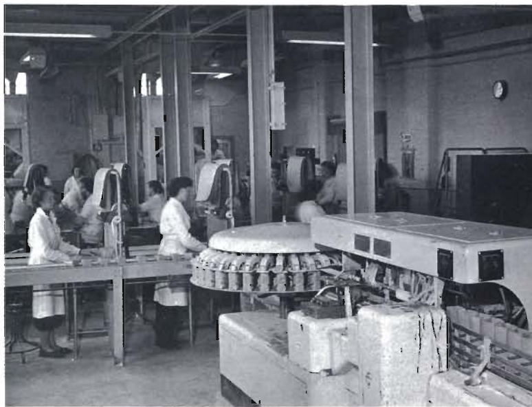
Plate 41. Machinery for filling sugar bags. (Section 15). PHOTO: British Sugar Corporation
