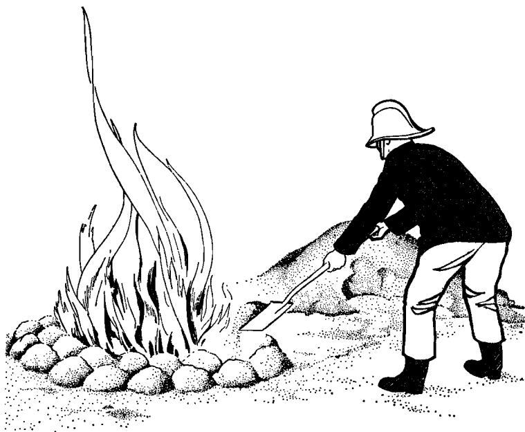
Fig. 27. Method of applying dry sand on to a metal fire.
