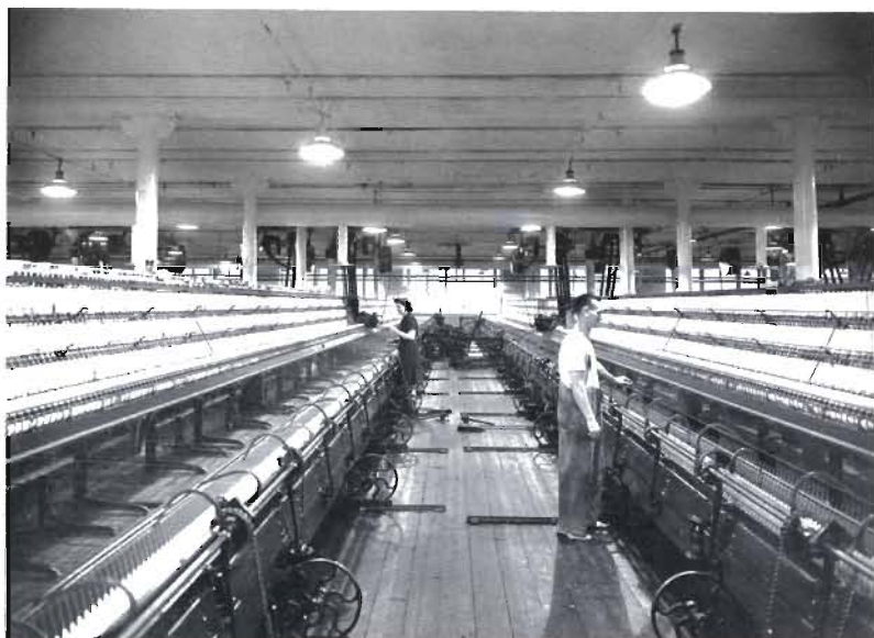
Plate 15. Spinning mules in a cotton mill, showing the lack of space between the mules when the carriages reach the end of the metal runways. Fire can spread with great rapidity along the mules. (Section 4).
