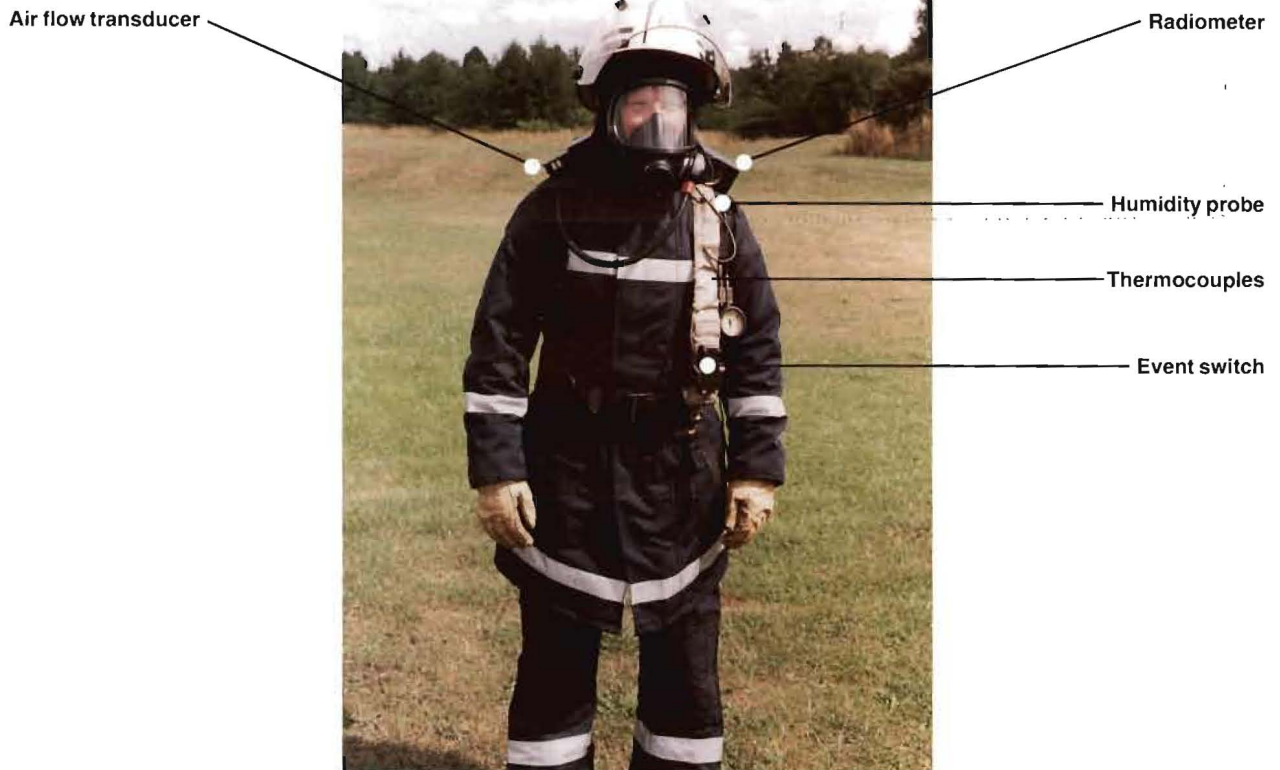
Figure 1: Package on BA wearer showing positions of the sensors.
