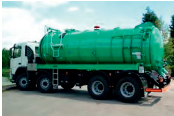
Vacuum-operated waste tank
