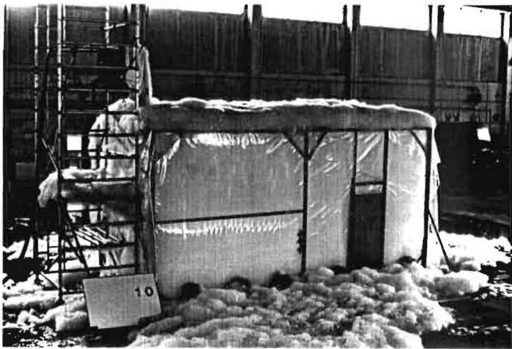
Figure 3 - The enclosure filled with high-expansion foam. C/615/84
