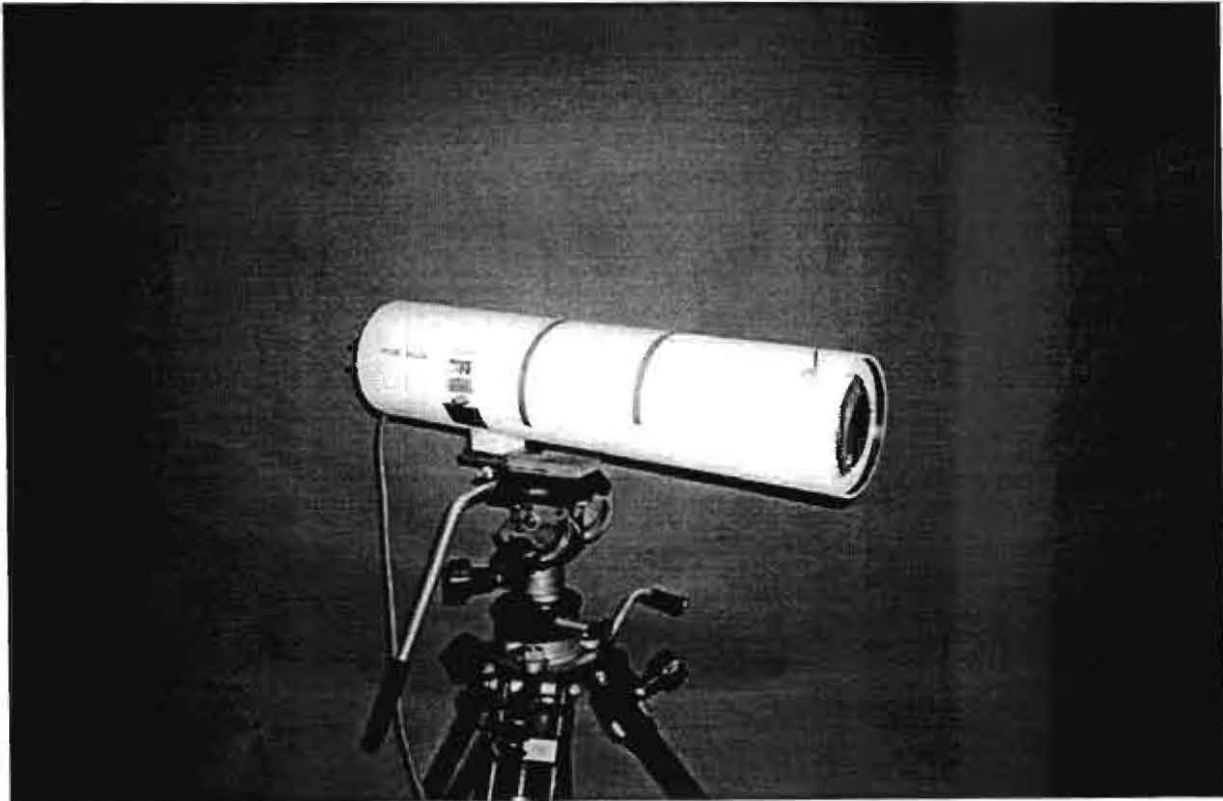
Figure 8: Spark gap device
