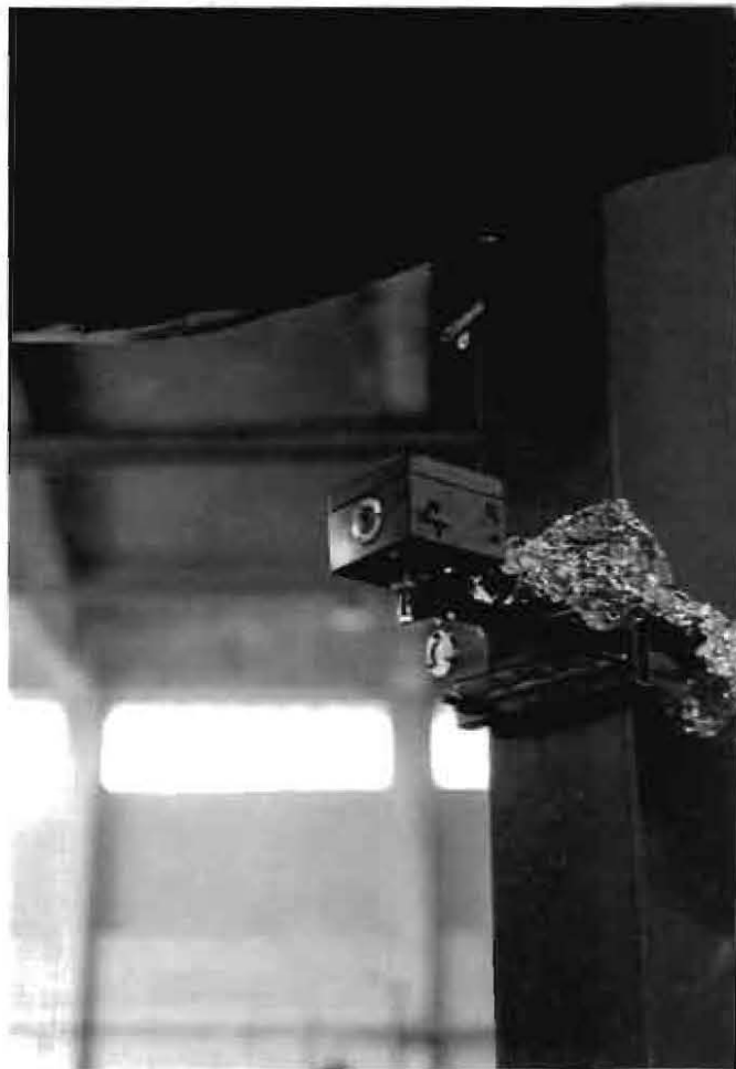
Figure 7: Radiometer positioned on a bracket clamped to a stanchion
