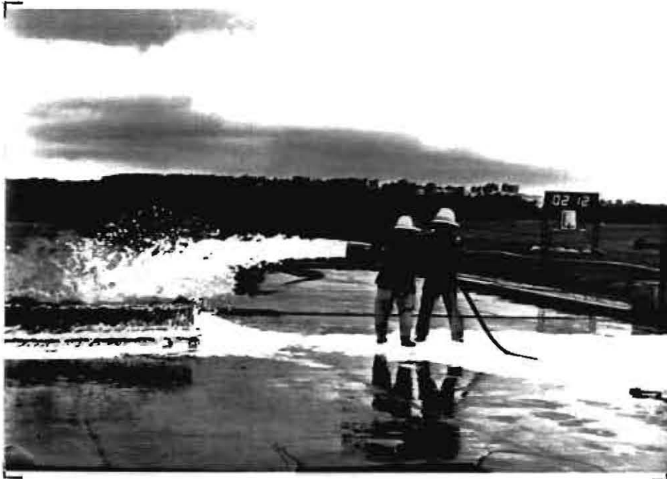
Figure 7: Application of medium-expansion (65) foam from KR2/75 branchpipe. (Test 4)
