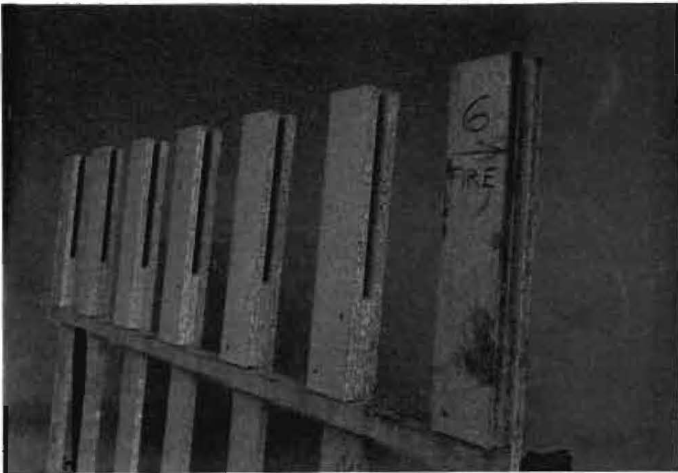
Figure 22 Fire Spread Witness Marks for Day 2 Test 2 (C226/1998)
