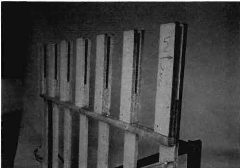
Figure 21 Fire Spread Witness Marks for Day 2 Test 1 (C231/1998)
