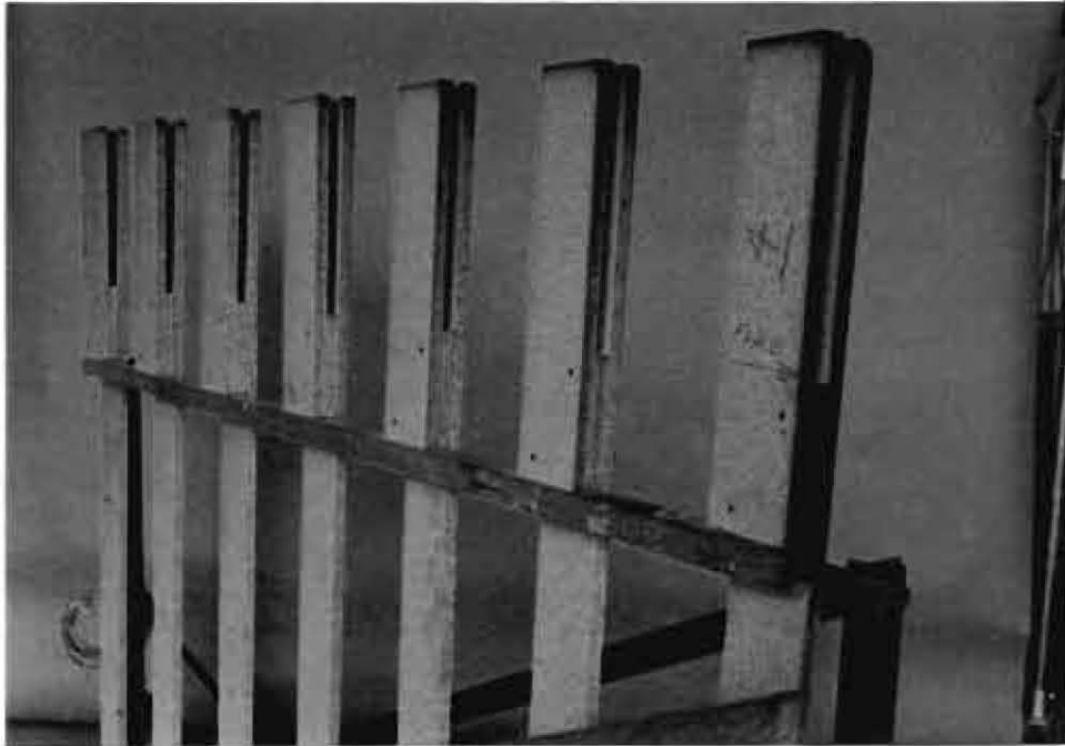
Figure 20 Fire Spread Witness Marks for Day 1 Test 4 (C238/1998)
