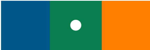
Figure 8: Example of a colour band for a 132kV tower - diagram courtesy of UK Power Networks
