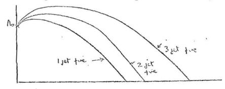
As the severity increases the amount of spread and control time also increase.
