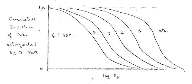
A fire of a given size can be characterised by its relative severity - ie a number between 0. and 100 which determines its position on the cumulative scale of numbers of jets required.
